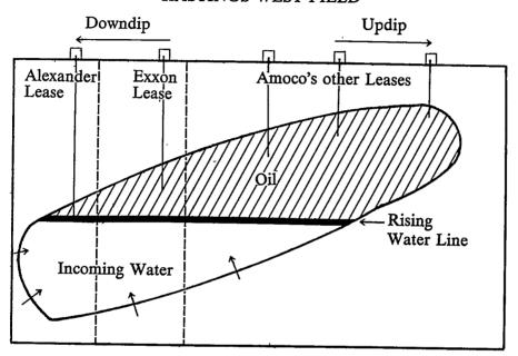
The combination of these two characteristics dictated that as oil was removed from the field, regardless of well location, incoming water forced the remaining oil towards the updip leases.<sup>31</sup> This regional migration toward the southeast resulted in the field-wide drainage of oil from beneath Alexander's land so that the wells on that lease would eventually produce only water.
